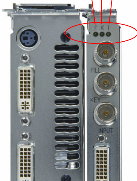
Figure 4.4 Connection Status Indicators - NVIDIA Quadro FX 5600
