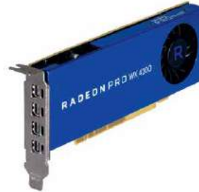
AMD RADEON PRO WX 4100 3.46 TFLOPS 4 GB Memory 4 Displays
