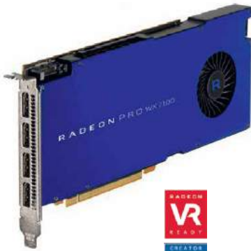
AMD RADEON PRO WX 7100 5.73 TFLOPS 8 GB Memory 4 Displays
