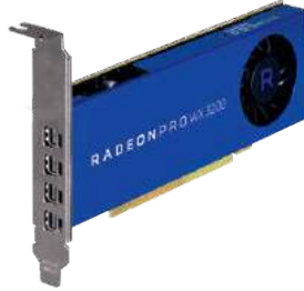
AMD RADEON PRO WX 3200 1.66 TFLOPS 4 GB Memory 4 Displays
