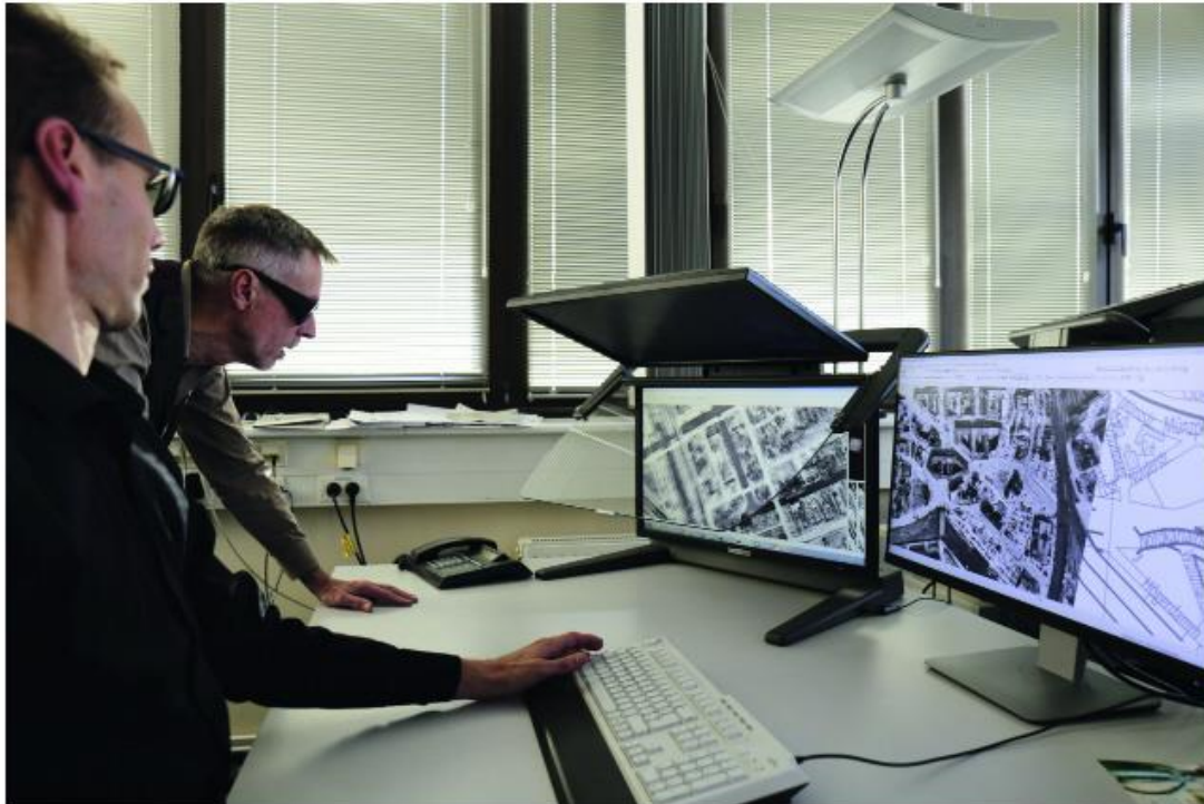
The high-resolution 3D PluraView displays (2,560 x 1,440 pixels) are completely integrated into the analysis process chain of the Hamburg Fire Brigade. The Hamburg Fire Brigade operates a total of 20 workstations with passive 3D-stereo monitors for the remote sensing of potential dangers.
