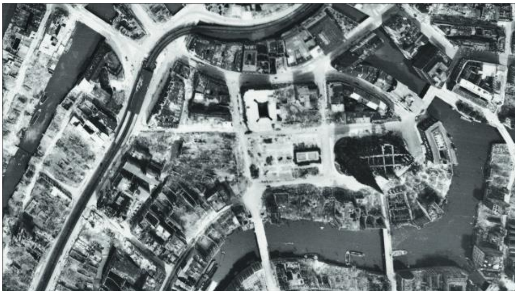
Working out what are suspected locations of unexploded bombs, and what are tree crowns or open manhole covers: With the utmost meticulousness, the Hamburg Fire Service interprets wartime aerial photographs to clarify whether or not there might be unexploded ordnance present. 3D stereoscopy helps to differentiate between small craters and mounds.
