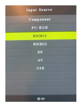
2 Using the remote control, select PC RGB, HDMI, or Video source to select your source. If desired source is not selected, press multiple times to toggle through the input options.
