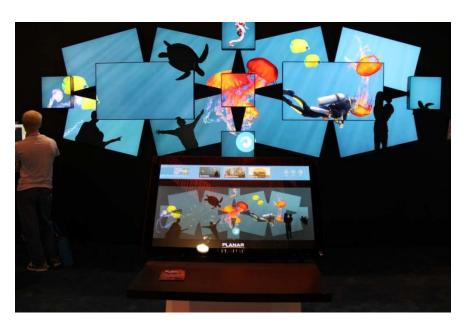
This interactive installation was designed for a trade show, but is applicable for a variety of museum, retail, and hospitality applications. The software, designed by IdentityMine, uses a small touchscreen (the top-rated Planar Helium 27") to control an artistic array of Planar Mosaic displays, in real-time. Users touch the small screen and the wall immediately responds.
