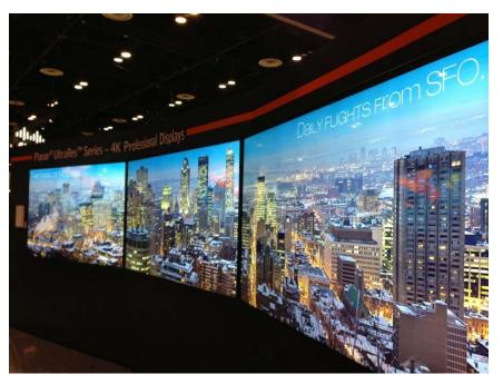
This three-wide configuration of <u>Planar UltraRes Series 4k displays</u> was built first for the InfoComm 2013 trade show and has been gaining popularity for conference and collaboration rooms. Delivering a whopping 12-times- HD resolution, this 19-foot wide wall is slightly faceted for an even more immersive feeling.
