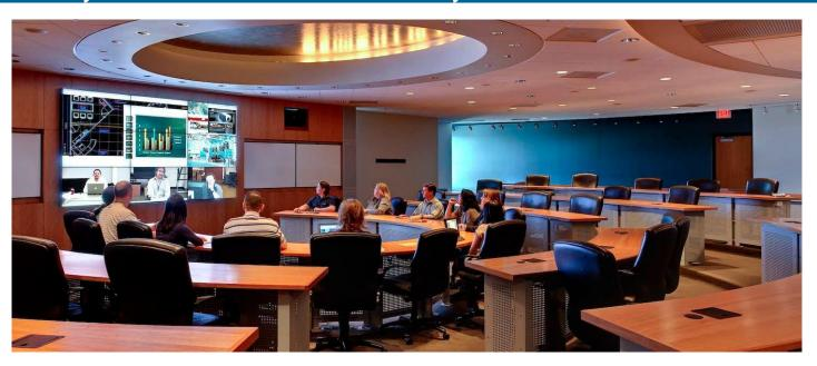
This executive board room is outfitted with a 3x3 array of <u>Clarity Matrix</u> to create a tiled LCD video wall. The displays add to more than 4k resolution, but the input is set to 4k to allow for high resolution images and video to be played. The room is controlled with a AMX touchscreen system and the <u>Clarity Matrix architecture</u> leaves the wall quiet and easy to service, with no power outlets behind the wall.
