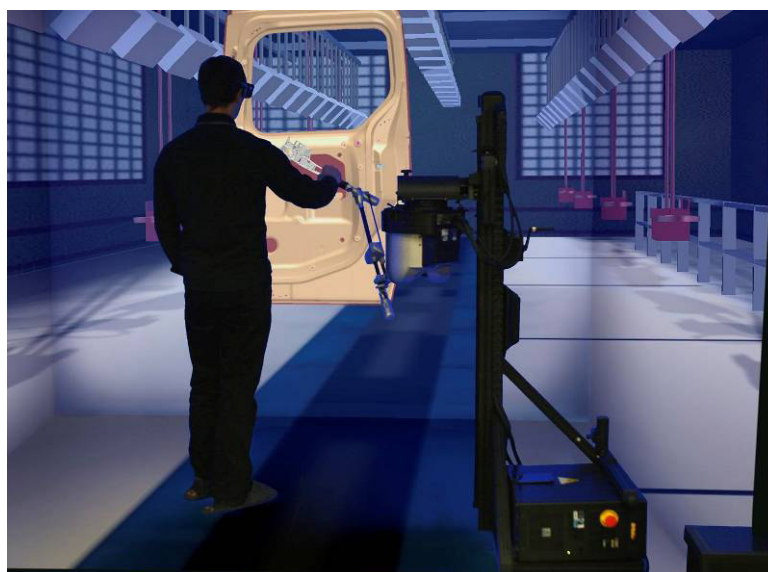
Assembly simulation inside a CAVE™ (picture © PSA Peugeot Citroën, France)
