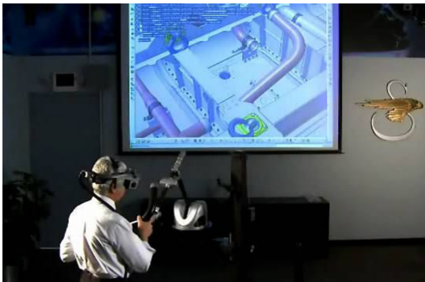
Assembly simulation of fuel lines inside a helicopter (picture © Sikorsky Aircraft, Stratford, CT, USA)
