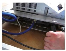
a. Remove all connecting cables (power, HDMI, network and USB).
