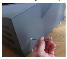
a. Loosen the two side panels on the corresponding projection housing (top or bottom) and then remove the side panel.
