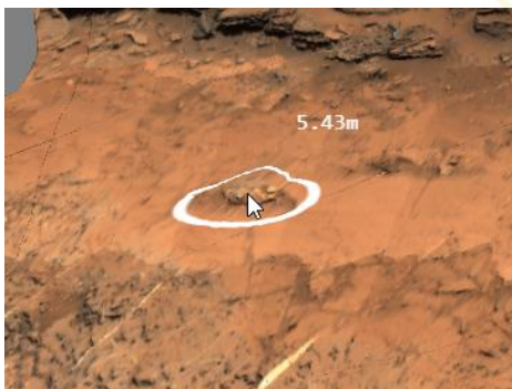
Figure 1: "Footprint Cursor" combined with the standard windows cursor Pro3D [7]. This approach is easily portable to 3D
