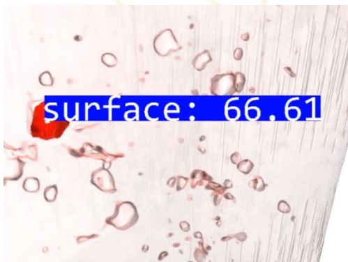
Figure 2: Billboard (3D) with selected pore of casting part in Aardworx Volume Renderer [8]. For 3D viewing the billboard should be placed at proper depth.
