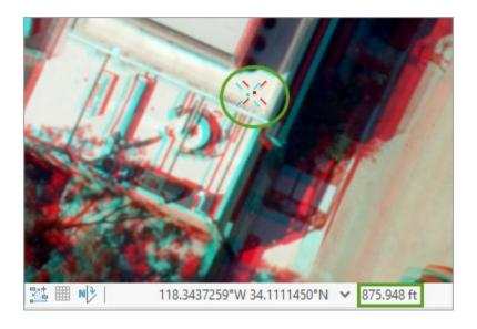
18. From the **Create feature** template, use the **Point** tool to create a second point on the lower terrace.
