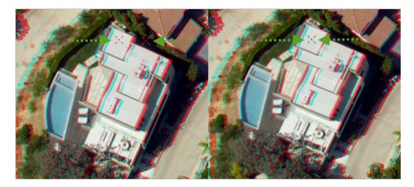
To increase the z-value, rotate the wheel button backward. To decrease the z-value, rotate the wheel button forward. You will have the correct height when the cursor appears to sit on top of the feature you are viewing, and the red and blue crosses come together.
