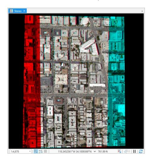
In the stereo map, the cursor always returns x, y, and z, which are displayed in the current projection units below the map.
