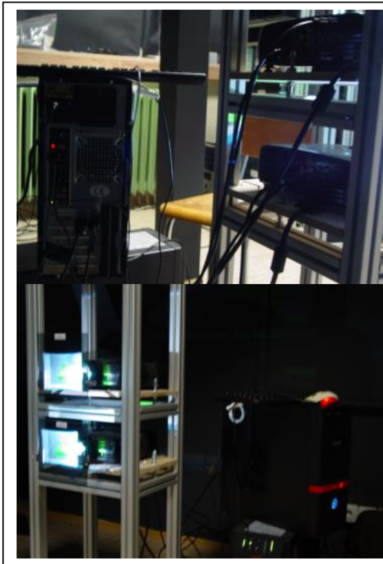
Fig. 10. Two beamers with passive polarization filters connected to the outputs of a quad-buffered graphics adapter
