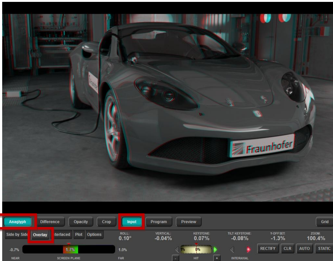
Figure 10: The Anaglyph Overlay mode can be used to get a visual feedback of the quality of the mechanical alignment. Red or cyan lines around horizontal object borders in the image are clear indicators of the presence of vertical disparities and thus a poor mechanical alignment.
