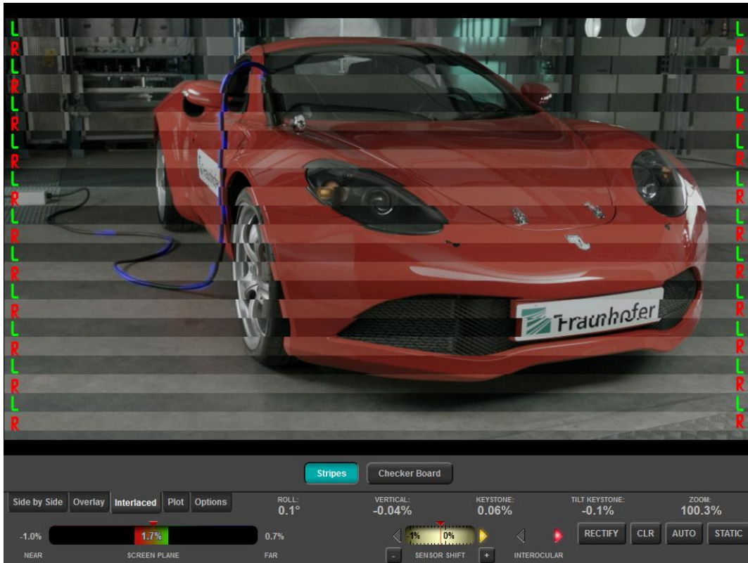
Figure 24: The Stripes visualization mode can be active in the Interlaced tab. Color and aperture differences are easy to recognize in this view mode. Additionally, you can find easily overview horizontal disparities in this view mode.
