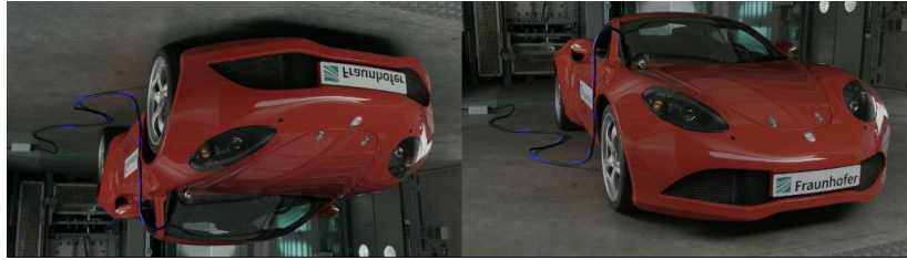
Figure 4: Unmodified camera signals. The left image is flipped due to the use of a mirror rig while shooting the content. Using the Side-by-Side view mode, one can easily perceive which flipping option is necessary.
